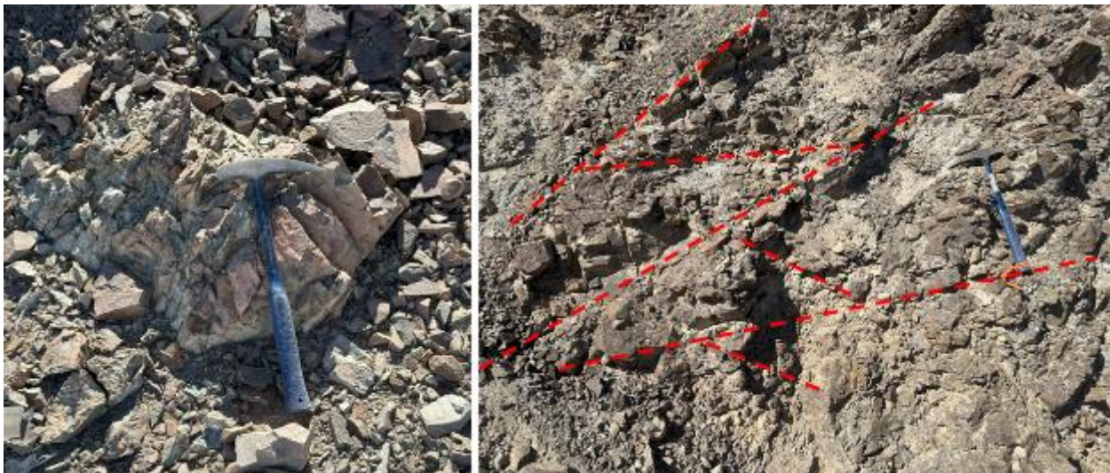
Figure 19: Left, Stockwork with limonites in diorite, with moderate argillic-chlorite alteration and presence of epidote. Right, Stockwork of quartz veinlets, strong argillic-chlorite alteration (In red, veinlets of quartz).
